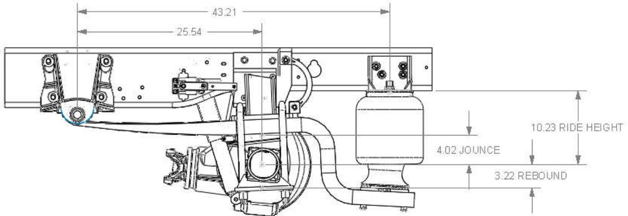
Note: The ride height is for the completed vehicle with body and components. See table below for correct vehicle dimensions. See following pages for the above views.
