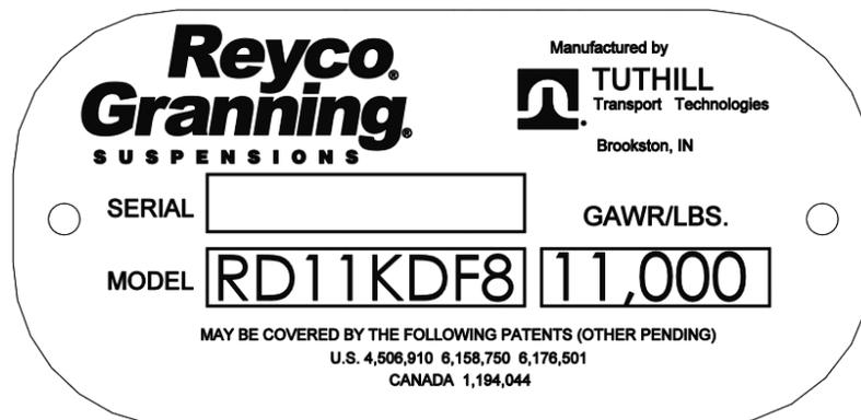
Figure 1: Suspension Identification
