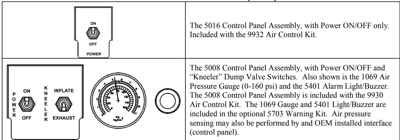
Operation of the ReycoGranning® *AIRGLIDE*® drive axle suspension utilizing an automatic height control system is reached through various control panels. Depending upon options included with the suspension system, the control panel should be operated as follows:
