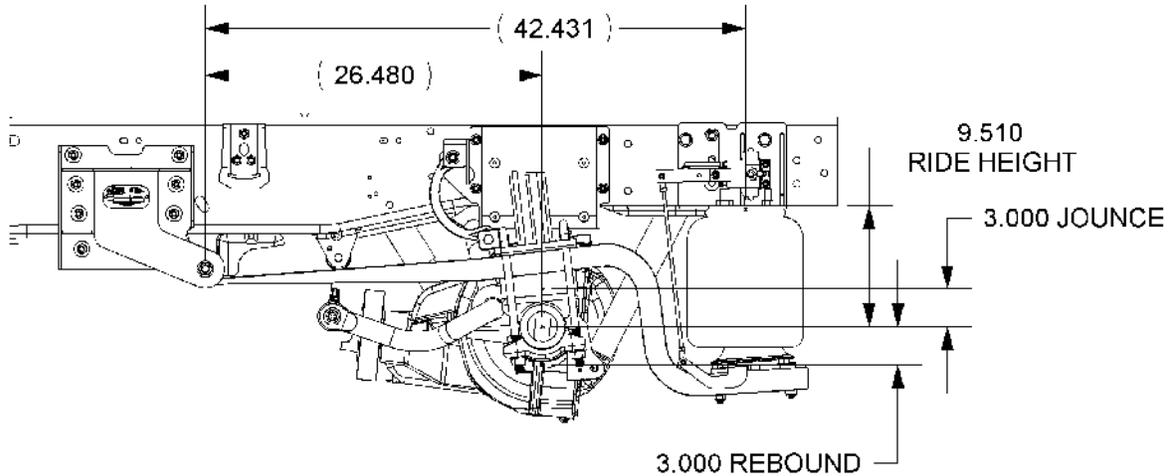
Note: The ride height is for the completed vehicle with body and components. See table above for correct vehicle dimensions.
